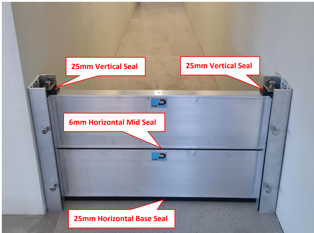
Figure 6 - FDD Sealing Mechanism
